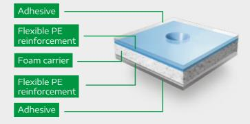
Equipped with a flexible, double-sided PE reinforcement for excellent print quality
