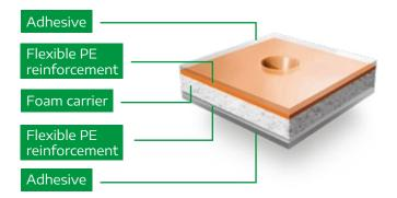
Equipped with a double-sided, flexible PE reinforcement for excellent print quality
